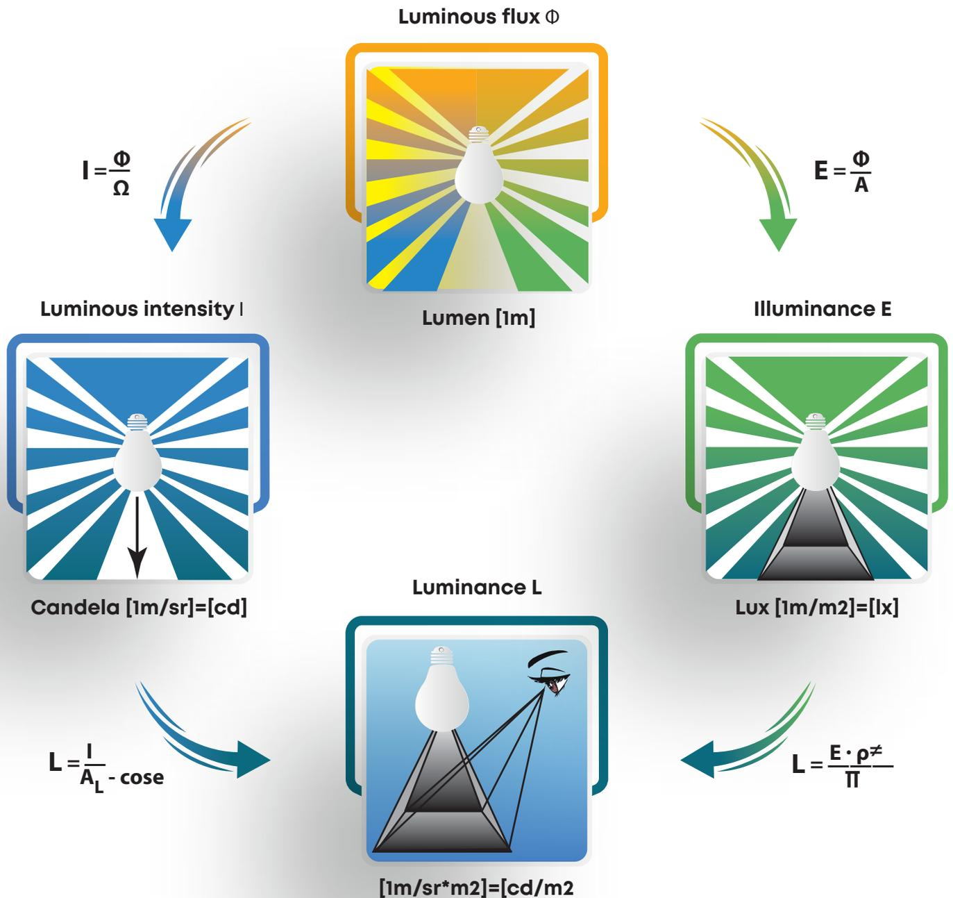
$\Omega$  = solid angle into which luminous flux is emitted
