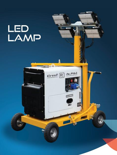
These vertical mast light towers come standard with an manual winch for easy deployment. Standard analog controls are easy to use and allow for individual light operation. Upgrade to the fully programmable Deepsea controller with auto start/stop and dusk-to-down sensor.
